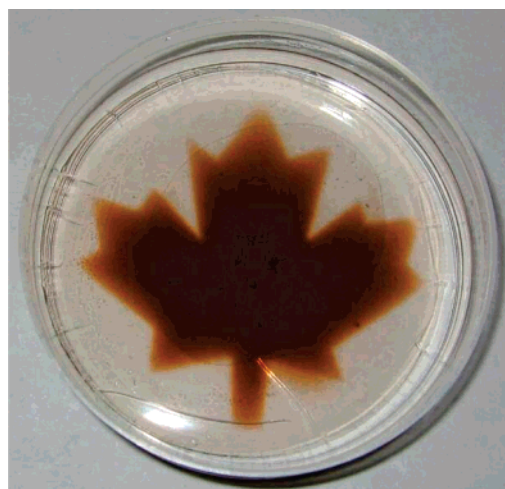
Figure 7. Selective irradiation of a circular slice of 2 ·SG with a black plastic maple leaf on top. The nonirradiated area is maroon, while the photolyzed area is colorless. Light source: 25 W tungsten bulb.
